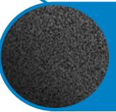
IKO has refused to reduce back coating from our shingles. Based on our experience, we believe that back coating adds to the overall asphalt content of the shingle which ensures long term weatherability and performance of our products.
